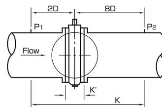
Flow coefficient based on K'
